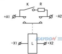
Single Pole Single Throv + Contactor. (One Normal Open) +A1.-A2 Main Contact Terminal -X1.+X2 Coil Terminal
