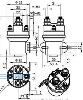
MW 平支架 螺丝接线 MW Flat support, thread
