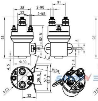
HW 圆弧支架 螺丝接线 HW Arc fixing method, thread
