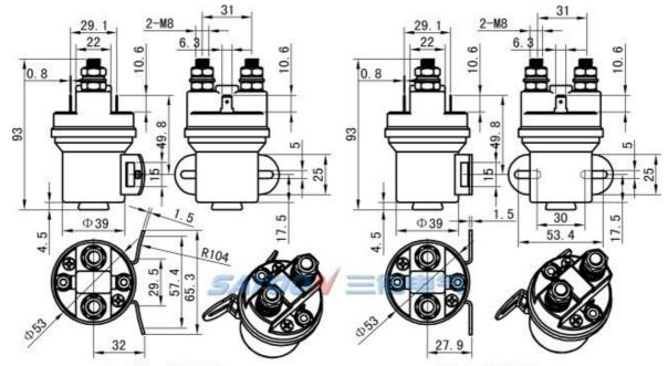
HP 圆弧支架 插片接线 HP Arc fixing method, Spade terminals
