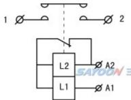
Single Pole Single Throw Contactor. (One Normally Open) 1.2 Contact Terminal A1.A2 Coil Terminal L1 Take-off the winding
